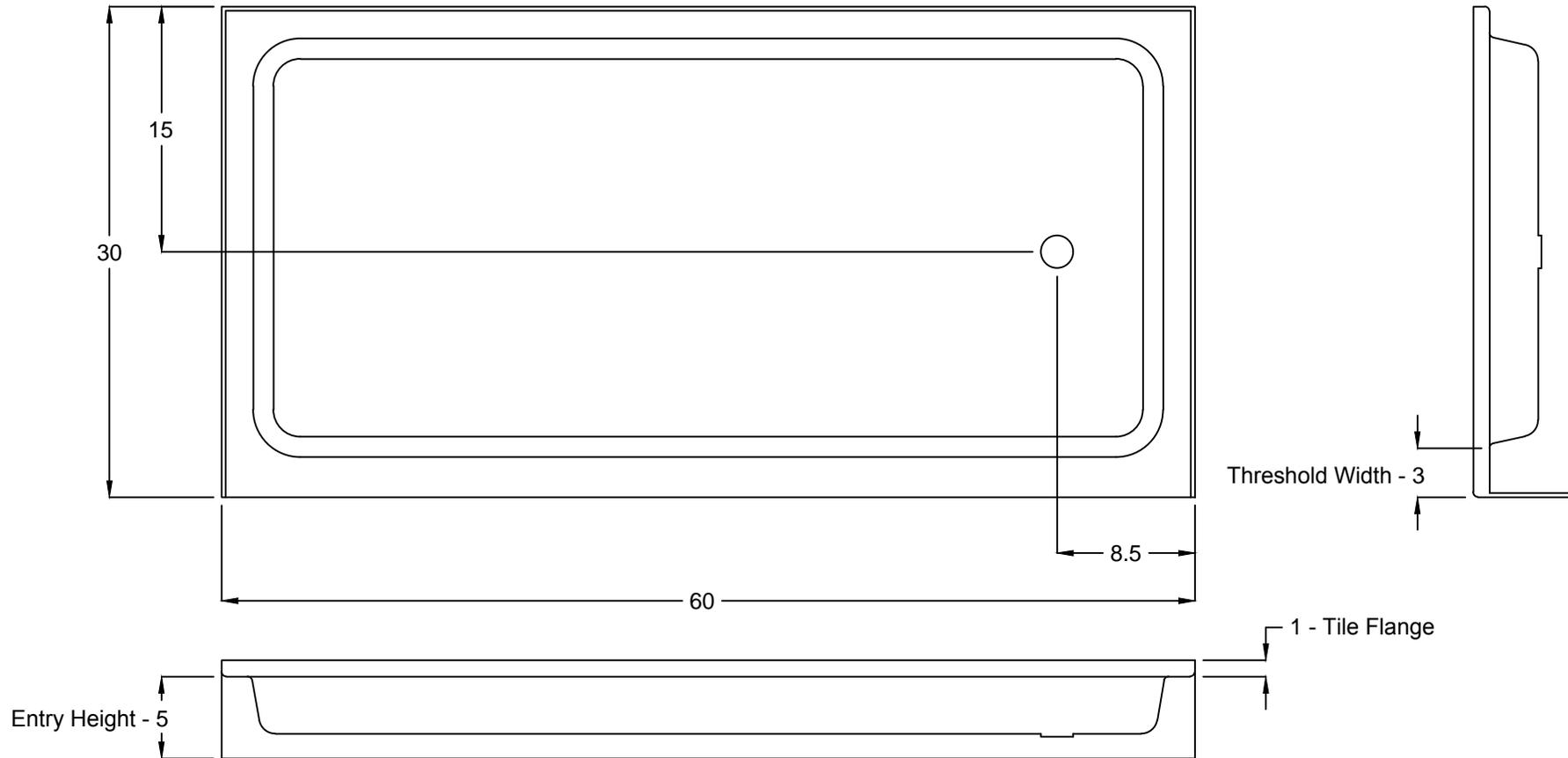
RH-Drain Shown. LH-Drain is mirror image.
