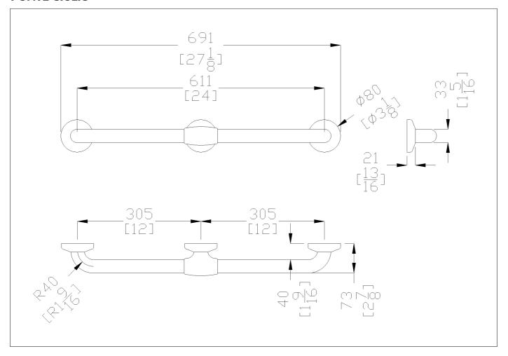
Bariatric 24" antimicrobial vinyl coated grab bar. No maintenance 3mm thick antimicrobial vinyl coating. Concealed stainless steel 11-hole flange plate.
