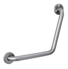
12"x12" angled grab bar. 1.25" diameter, 1.2mm wall thickness, 304 stainless steel.
