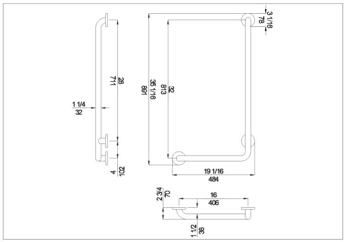
16"x32" stainless steel L-shape grab bar with concealed flange plates, right handed orientation. 1.25" diameter, 1.2mm wall thickness, 304 stainless steel.
