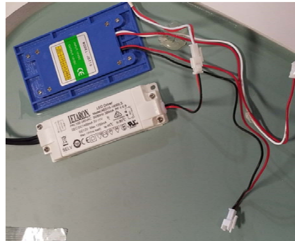
Touch Sensor By-passed for Wall Switch operation
