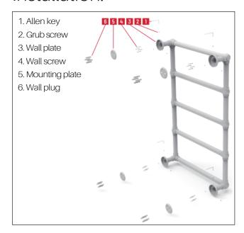
**Step 1:** Select the desired mounting position, make sure the wall is adequate to take the fixing points of the rail i.e anchor points must be securely attached to a stud or masonry.
